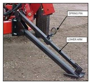
**Figure 5.3 Outrigger Work Position**
